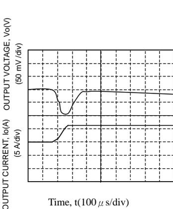
Fig.1 Typical Transient Response to Step Load Change from 0% to 100% of Io, max at Room Temperature and 5V Input (Waveform Averaged to Eliminate Ripple Component.)
